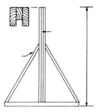
This upright consists of two pieces 1" x 3" and one piece 1" x 2", nailed together, with the 1" x 2" forming the groove for the boards to slide in.
