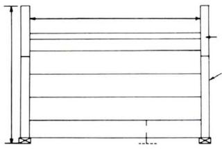
These boards are removable FRONT VIEW SIDE VIEW 1" x 3" brace groove top view of groove This upright consists of two pieces 1" x 3" and one piece 1" x 2", nailed together, with the 1" x 2" forming the groove for the boards to slide in. 5' - 0" 1" x 3" 1" x 3" 2" 4" 8" 8" 8" 8" 4' - 0" 4' - 0"
